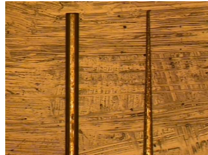
0.3mm electrode before & after cutting with de-ionised water
